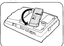
To temporarily place the handset down during a conversation, hook as shown.
